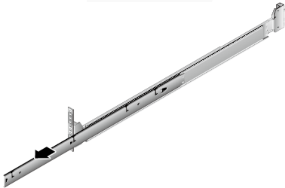
Figure 7-10 Pulling out an inner rail
