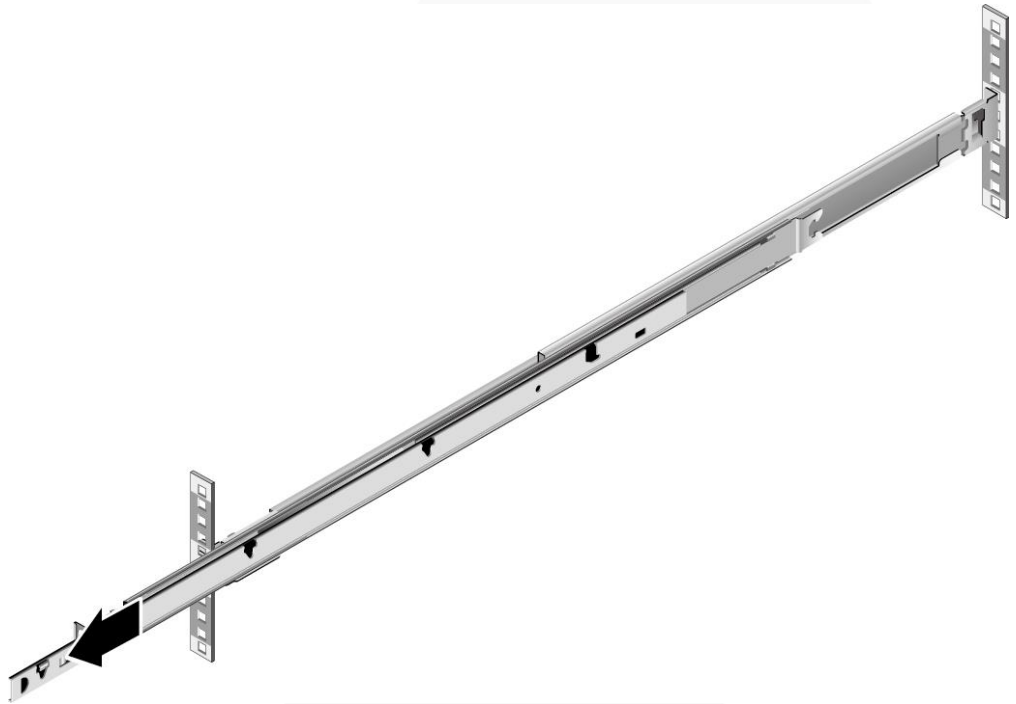
Figure 7-14 Pulling out an inner rail
