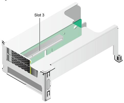
Figure 5-52 PCIe riser module 6
