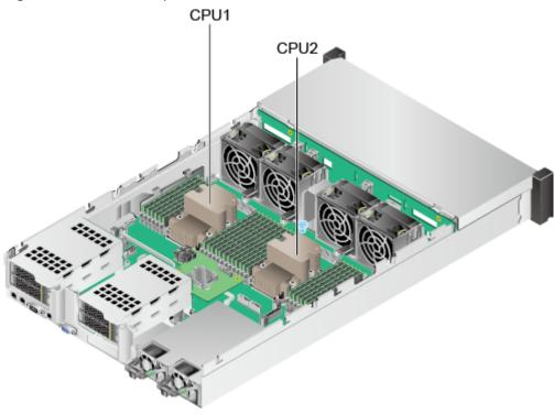
Figure 5-19 Processor positions
