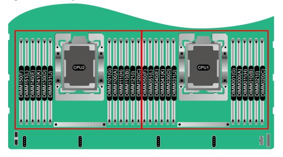
Number of DIMMs (√: recommended o: not recommended) **CPU** Channel **DIMM Slot** 0 ✓ 0 1 2 3 4 5 6 7 8 9 10 11 12 DIMM000(A) A DIMM001(G) DIMM010(B) В • DIMM011(H) DIMM020(C) C DIMM021(I) CPU 1 DIMM030(D) D DIMM031(J) • • • • DIMM040(E) E DIMM041(K) • DIMM050(F) F DIMM051(L)
