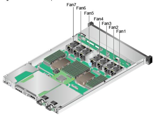
Figure 5-32 Fan module positions
