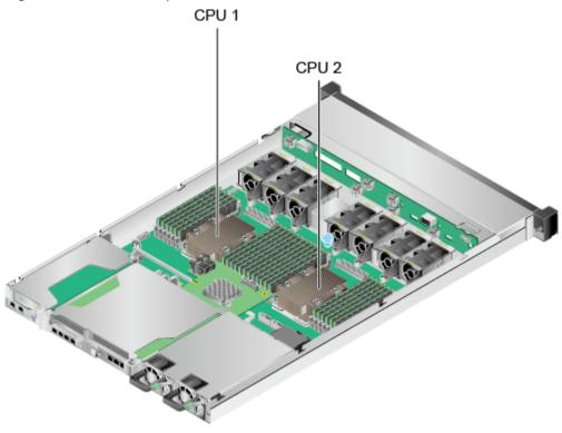
Figure 5-13 Processor positions
